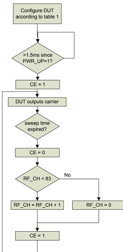
Figure 2. TX carrier wave sweep test routine
