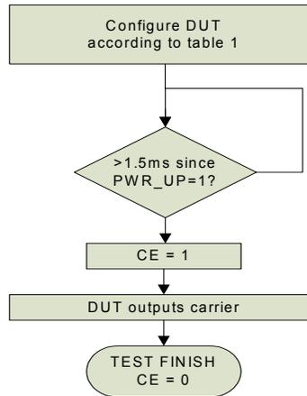
Figure 1. TX carrier wave output test routine
