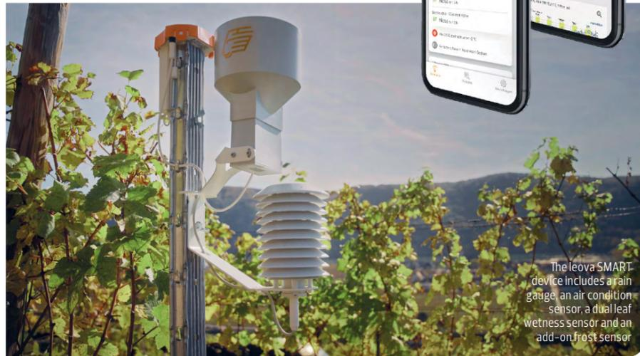
The leova SMART device includes a rain gauge, an air condition sensor, a dual leaf wetness sensor and an add-on frost sensor.
