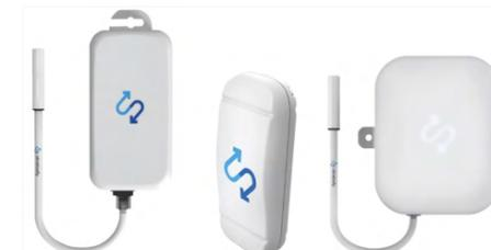
surface temperature of front- and back-of-house equipment. The Nordic SoC enables the temperature data to be wirelessly relayed via Bluetooth 5 connectivity to the gateway.
