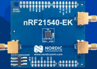
*The nRF21540 DB is a dual-kit development bundle for the nRF21540 RF front-end module, enabling range extension on all nRF52 and nRF53 Series SoCs.*
