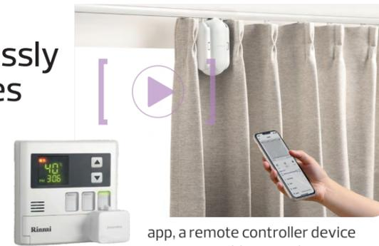
app, a remote controller device or a compatible smart home ecosystem such as Amazon Alexa, Apple Siri and HomePod or Google Home. Using the functionality of its built-in sensors, the device can be scheduled to close curtains at night and open curtains when it senses daylight.
