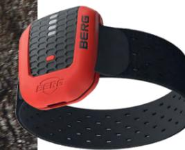
BERG AirHive developed by WRLDS Creations can achieve a playtime of at least one week between charges, made possible in part due to the ultra low power characteristics of the Nordic SoC. Jump data is relayed from the device to the BERG AirHive app on the user's smartphone using the SoC's Bluetooth LE wireless connectivity. The app includes minigames, skill training, jump analytics and a social flow function which allows users to upload their latest tricks and create challenges for others
