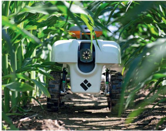
Autonomous robots fitted with cameras and sensors can be deployed in fields to monitor crops for any sign of disease or pest infestation
