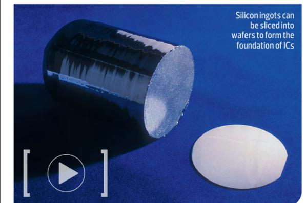
Silicon ingots can be sliced into wafers to form the foundation of ICs
