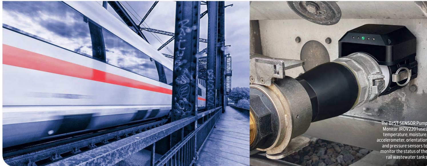
The BeST SENSOR Pump Monitor JROV2201 uses temperature, moisture, accelerometer, orientation and pressure sensors to monitor the status of the rail wastewater tanks
