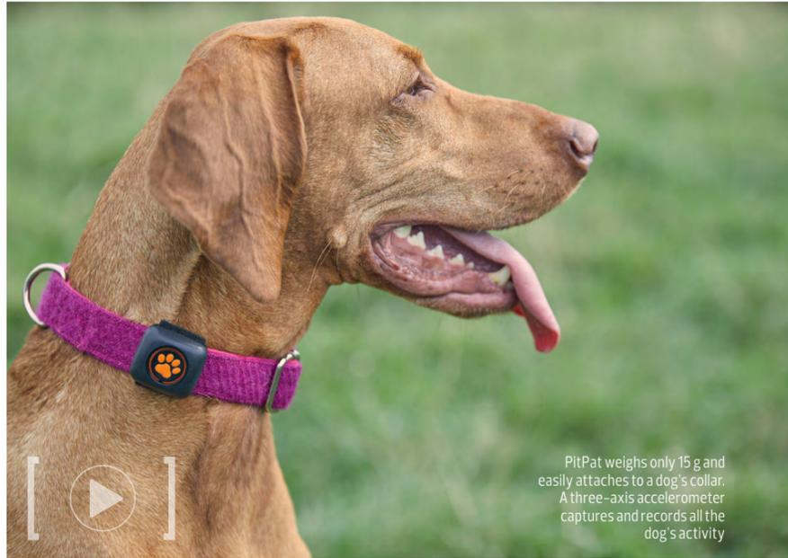
PitPat weighs only 15 g and easily attaches to a dog's collar. A three-axis accelerometer captures and records all the dog's activity
