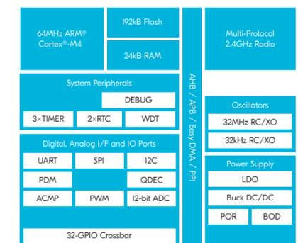
The nRF52811 supports Bluetooth 5.2, 802.15.4, Thread and 2.4 GHz proprietary. The nRF52811 offers a good option for a network processor and when paired with a companion microprocessor is a high value proposition for smart home gateway and router applications.
