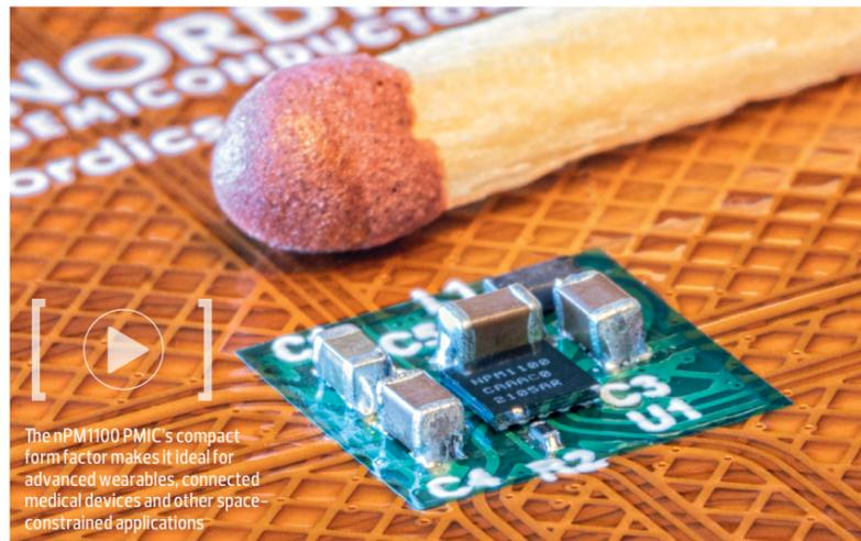
The nPM1100 PMIC's compact form factor makes it ideal for advanced wearables, connected medical devices and other space-constrained applications
