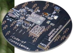
The original hardware for Code of Conscience was based on the Nordic Thingy:91 multi-sensor cellular IoT prototyping platform. The open source software provides the GPS-based geofence capabilities which interlock with the fuel pump systems of heavy machinery, enabling automatic shutdown if the equipment moves into a restricted area. Integrated cellular connectivity enables notifications and audits of the machinery's position. (See [WQ Issue 3, 2020](#) pg10.)
