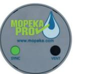
Mopeka's Pro Check Sensor mounts underneath a cylinder and uses ultrasound to inform the user how much fuel is left
