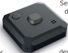
periodically transmits its unique identifier for receiving devices to monitor and then measure the difference in 'Time of Flight' (ToF) between the Bluetooth LE packet and an ultrasonic audio signal. The time difference is proportional to the distance between transmitter and receiver.
