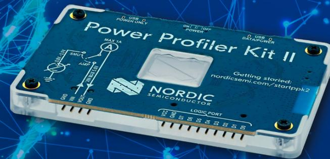
Enables easy and affordable power measurements for wireless product development on all Nordic DKs, in addition to external hardware.
