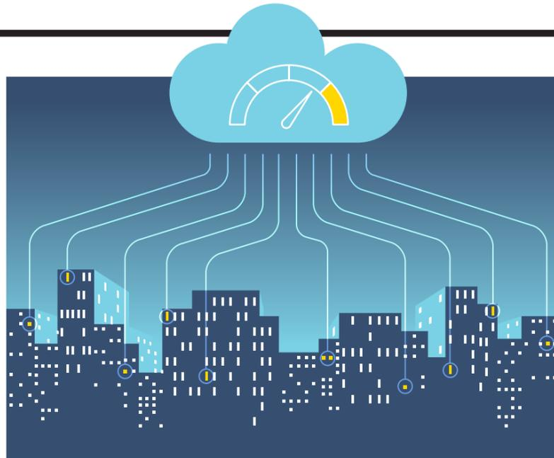
floors of a large apartment building. Metering data is sent to the Lobar Platform in the Cloud, where it gets parsed, displayed and made available for further processing. It is also possible to use the Lobar gateway without the platform and instead connect it to a standalone backend (as long as the backend is capable of parsing and decrypting wMBus 'telegrams').
