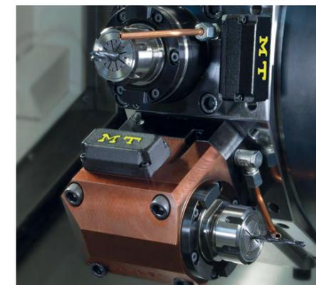
By using cellular IoT, InnBlue says the need for a gateway is eliminated. Encrypted data is sent periodically to summarize how a toolhead has been used, and automatically in the event of an alarm.
