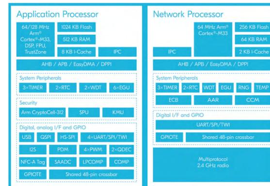
The nRF5340 features one Arm M33 processor optimized for performance and a second for efficiency. Both are accessible to the developer
