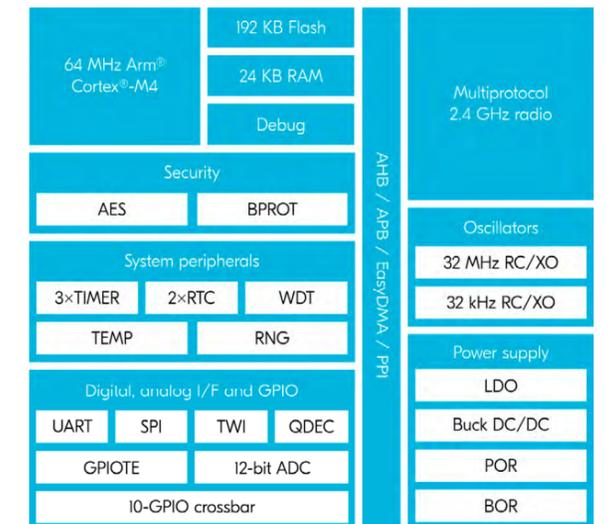
The nRF52805 SoC incorporates a 64 MHz 32-bit Arm Cortex M4 microprocessor, 192 KB Flash and 24 KB RAM, multiprotocol 2.4 GHz radio, power supply, peripherals and a range of interfaces in a 2.48 by 2.46 mm WLCSPP.
