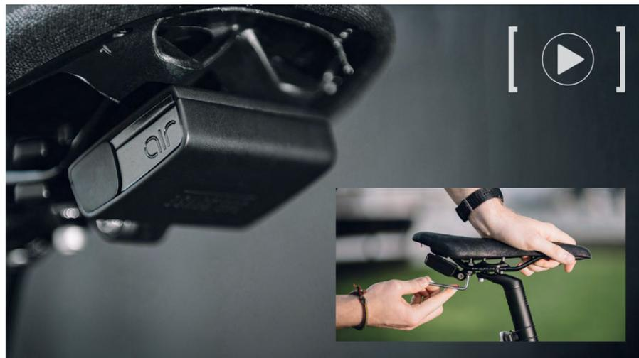
AIR will not only protect the bike, it will also protect its rider, identifying if the bike's been involved in a crash and sending an SMS with the precise location to the rider's assigned contact.
