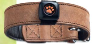
PitPat weighs only 15 g and easily attaches to a dog's collar. A three-axis accelerometer tracks the dog's motion throughout the day, and proprietary algorithms interpret this data to identify five specific activity states—walking, running, playing, pottering and resting—and how long the dog spends in each state
