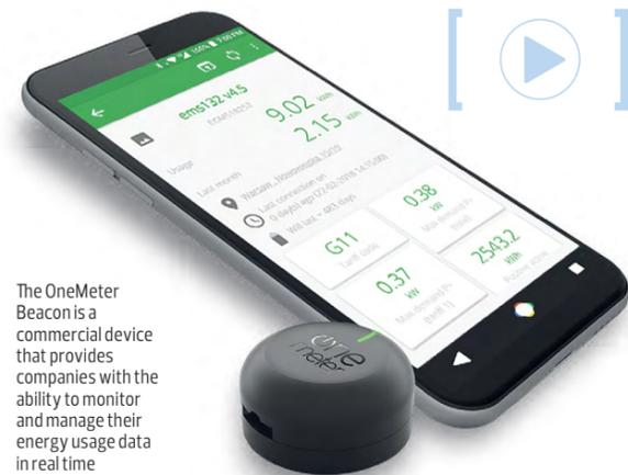
The OneMeter Beacon is a commercial device that provides companies with the ability to monitor and manage their energy usage data in real time
