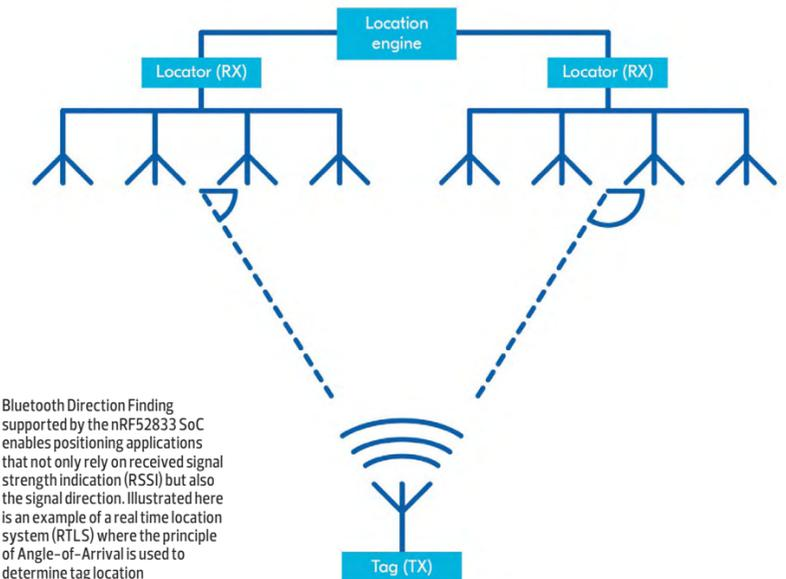
Bluetooth Direction Finding supported by the nRF52833 SoC enables positioning applications that not only rely on received signal strength indication (RSSI) but also the signal direction. Illustrated here is an example of a real time location system (RTLS) where the principle of Angle-of-Arrival is used to determine tag location
