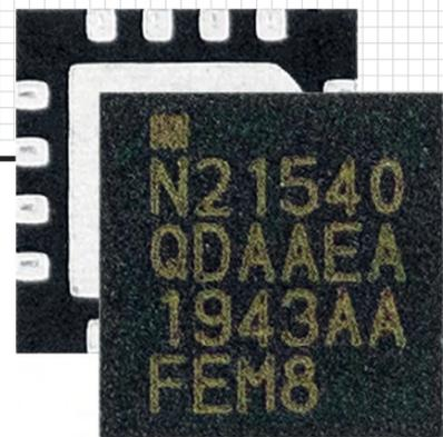
Nordic's short-range wireless SoCs. The nRF21540 connects to the SoC's antenna output and features two additional antenna ports to enable antenna diversity features. The device's gain control, antenna switching and power modes are controlled via GPIO or SPI or a combination of both.
