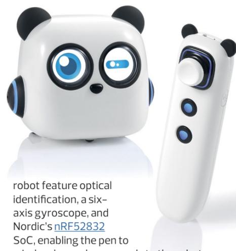
robot feature optical identification, a six-axis gyroscope, and Nordic's [nRF52832](#) SoC, enabling the pen to wirelessly send commands to the robot over Bluetooth LE connectivity, up to a range of approximately 10 meters in open areas.
