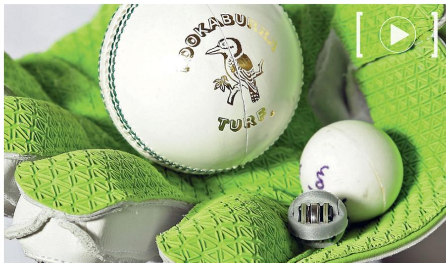
As soon as the movement data is gathered by the built-in sensors, relevant information is transmitted via the Nordic SoC enabled Bluetooth LE link to an iOS compatible app.
