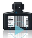
When traveling with a partner airline, passengers can check in remotely via the airline's smartphone app, and the flight information is then sent to and displayed on the smart luggage tag using Bluetooth LE wireless connectivity enabled by Nordic's [nRF52840](#) SoC. Once at the airport, users are then able to drop off their luggage without needing to use a check-in kiosk. Users can also track their bags throughout the airport handling process via the airline app.
