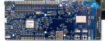
The nRF9160 SiP is also available on a powerful single-board DK made for the IoT application developer. The [nRF9160 DK](#) comes with free development tool support, [nRF Connect for Cloud](#) demonstration platform and the [nRF Connect SDK](#) in GitHub with sample applications.
