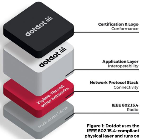
**Figure 1: Dotdot uses the IEEE 802.15.4-compliant physical layer and runs on Thread’s IP-based platform**
