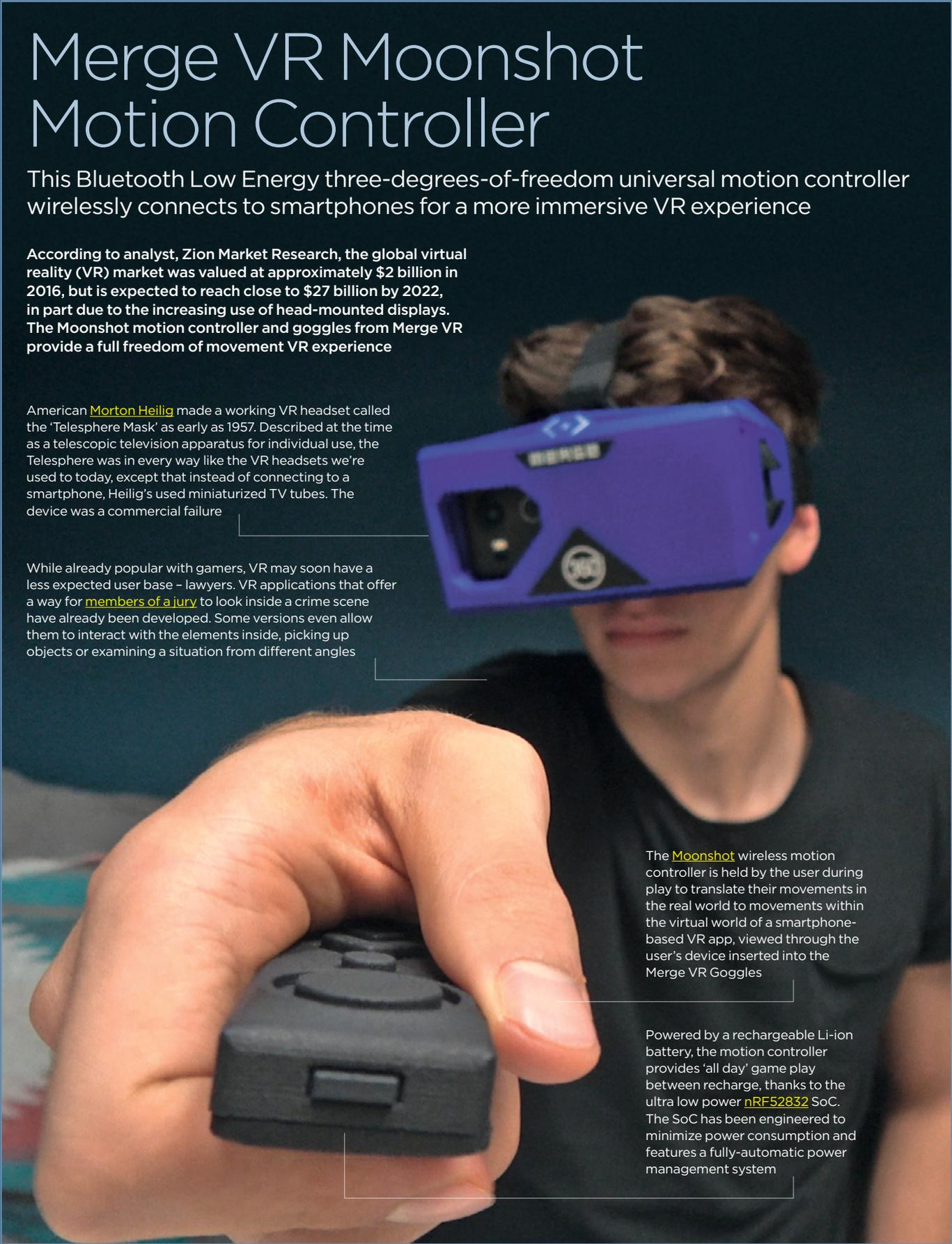
The [Moonshot](#) wireless motion controller is held by the user during play to translate their movements in the real world to movements within the virtual world of a smartphone-based VR app, viewed through the user's device inserted into the Merge VR Goggles
