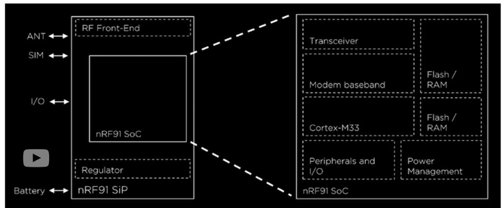
**The nRF91 Series SiP has been jointly developed by Nordic's experienced cellular design team in Finland and its low power wireless experts in Norway. The SiP comprises RF front-end, nRF91 Series SoC, and regulator**
