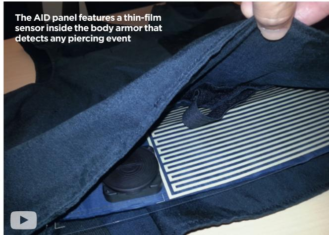
The AID panel features a thin-film sensor inside the body armor that detects any piercing event
