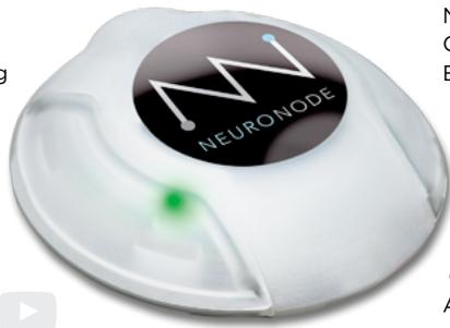
NeuroNode interprets signals sent from the brain to a muscle and uses EMG signals to control the user's paired device
