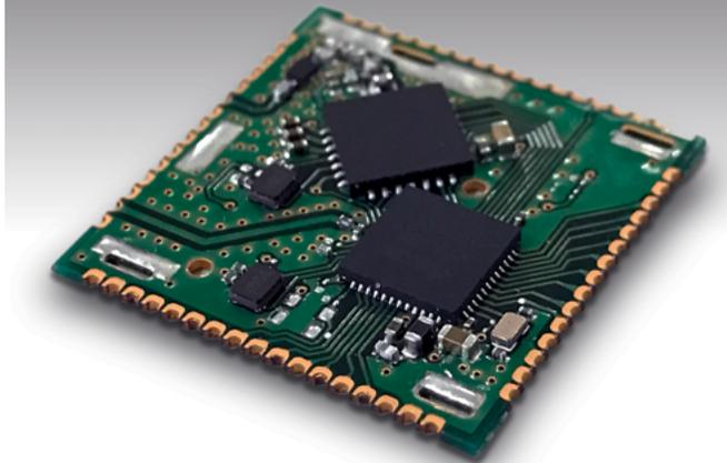
LoRaWAN application software. The module also features an integrated LoRaWAN RF chip—supervised by the nRF52832 SoC's embedded ARM Cortex M4F processor—for IoT wireless communication across LPWANs.
