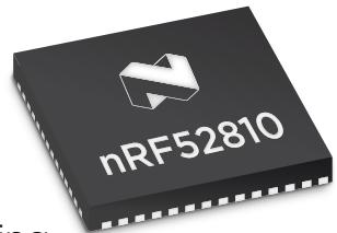
5-compliant RF protocol software 'stack' offering up to 20 concurrent links in a combination of Bluetooth low energy roles. The nRF52 Series' software architecture separates the protocol stack from the application software, allowing developers to quickly build, test, and verify application code with no risk of corrupting the stack.
