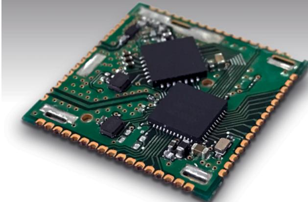
LoRaWAN application software. The module also features an integrated LoRaWAN RF chip—supervised by the nRF52832 SoC's embedded ARM Cortex M4F processor—for IoT wireless communication across LPWANs.
