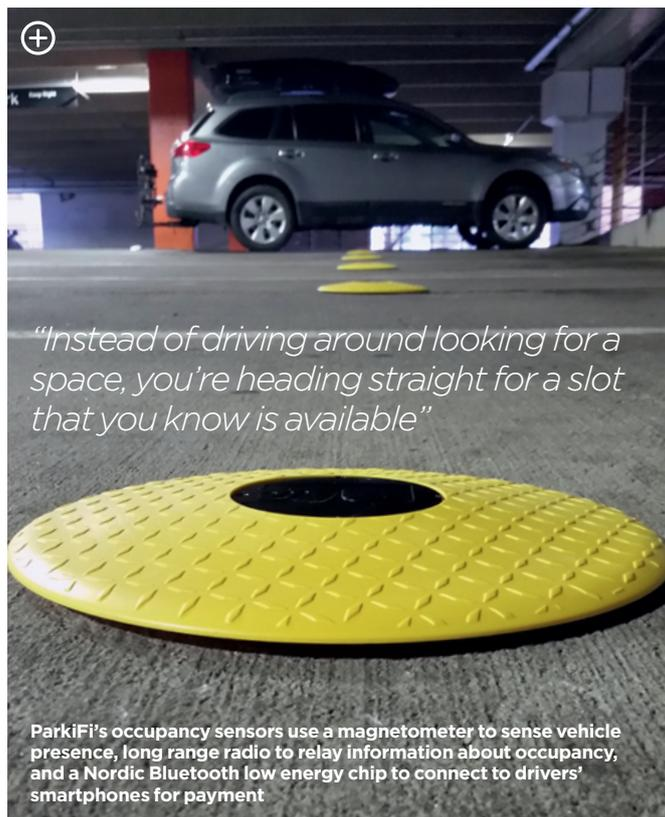
**ParkiFi’s occupancy sensors use a magnetometer to sense vehicle presence, long range radio to relay information about occupancy, and a Nordic Bluetooth low energy chip to connect to drivers’ smartphones for payment**
