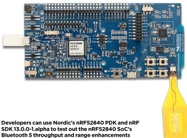
**Developers can use Nordic's nRF52840 PDK and nRF SDK 13.0.0-1.alpha to test out the nRF52840 SoC's Bluetooth 5 throughput and range enhancements**
