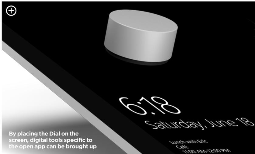
By placing the Dial on the screen, digital tools specific to the open app can be brought up
