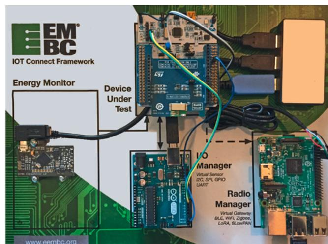
**EEMBC’s IoT Connect framework comprises an energy monitor, a radio manager to coordinate communication, and an IO manager to synchronize activities and to simulate a sensor input**
