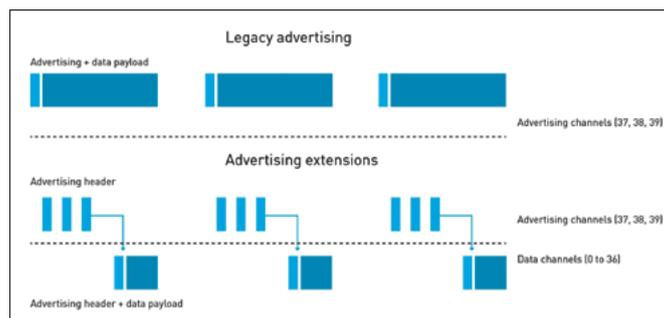
**Figure 1: Prior to Bluetooth 5, advertising packets were limited to the technology's three advertising channels. Busy use risked congestion. With advertising extensions, advertising data packets can be offloaded to normal data channels acting as secondary advertising channels**
