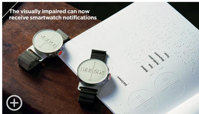
Two touch sensors allow the user to scroll through and read each notification, while two buttons and the “Dot Crown” dial operate the various functions available on the 43-mm diameter wearable
