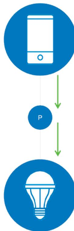
**Figure 2: Proxy Nodes (“P”) allow Bluetooth low energy devices that don’t support Bluetooth mesh (for example, smartphones) to connect to a Bluetooth mesh network**
