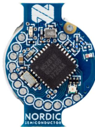
**Nordic's PoC PCB is based on the company's baseline nRF52810 and S112 SoftDevice making it an ideal reference design for inexpensive, disposal medical products**
