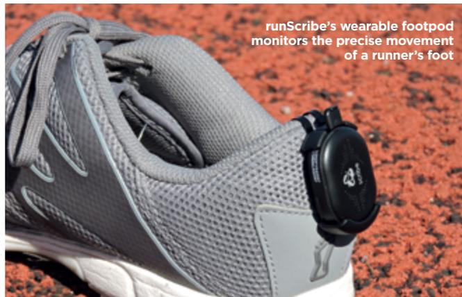
runScribe’s wearable footpod monitors the precise movement of a runner’s foot
