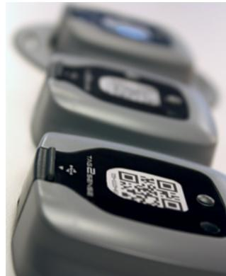
**A Tag2Sense asset tracking data logger contains five sensors to monitor the environmental conditions experienced by shipments in transit**
